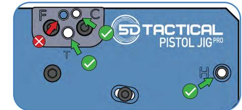
**DRILL THE 4MM HOLE LABELED "T" FOR TRIGGER, 3MM HOLE LABELED "H" FOR HOUSING, AND 3MM HOLE LABELED "C" ON THE DRILL GUIDE. FLIP JIG OVER AND REPEAT FOR OTHER SIDE.**
