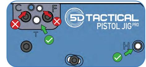
**S-10 IMPORTANT! Pinhole location is critical to the function of the frame and will cause issues if drilled incorrectly.**
